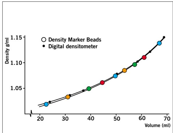
**Figure 15.** Correlation of recorded densities of a Percoll gradient in 0.15 M NaCl using Density Marker Beads and a digital densitometer (DMA 46, Anton Paar A.G.). Fraction size 2.64 ml, centrifuge MSE Superspeed 75, rotor 10 x 100 ml, angle 18°, 40,000 x g for 60 minutes. (Work from Amersham Biosciences, Uppsala, Sweden.)
