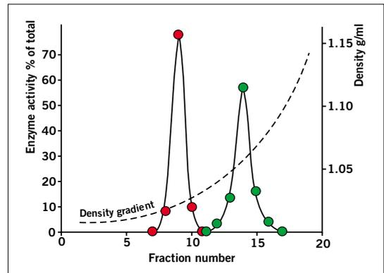
**Figure 7.** The density distribution of mitochondria from rat liver cells after incubation in iso-osmotic buffer (red) and buffer containing 17.5% albumin (green). Centrifugations were performed in a Beckman 65 rotor ( $23^\circ$  angle) for 30 minutes at  $40,000 \times g$ . (59, reproduced by kind permission of the authors and publisher).
