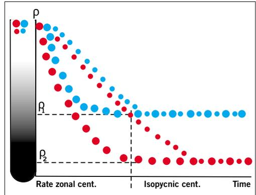
Figure 1. Diagrammatic representation of rate zonal and isopycnic centrifugation.  $\rho_1$  = buoyant density of the less dense (blue) particles  $\rho_2$  = buoyant density of the more dense (red) particles (Courtesy of H. Pertoft, reproduced by kind permission.)
