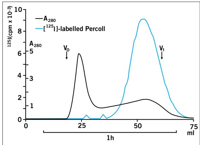
**Figure 18.** Gel filtration of microsomes obtained from gradients of Percoll containing <sup>125</sup>I-labelled Percoll on Sephacryl S-1000 Superfine. V<sub>o</sub> = void volume, V<sub>t</sub> = total volume. (275, reproduced by kind permission of the authors and publisher).
