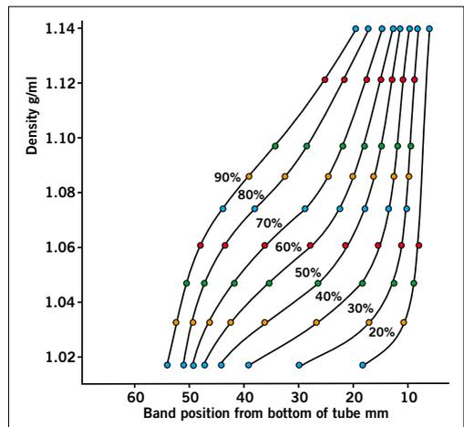
Figure 10. Use of colored Density Marker Beads to show gradient shapes. Dilutions of Percoll as in Figure 9, running conditions: 23° angle-head rotor, 60,000 x g, 15 minutes. Steeper gradients were formed by the greater g-force. (Work from Amersham Biosciences, Uppsala, Sweden.)
