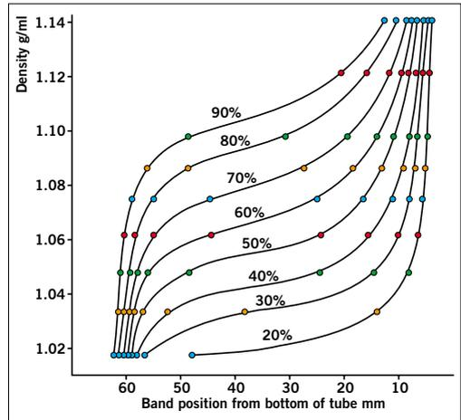
Figure 9. Use of colored Density Marker Beads to show gradient shape. Gradients formed from solutions of Percoll varying from 90% to 20% of stock isotonic Percoll in 0.15 M NaCl. Running conditions 23° angle-head rotor 30,000 x g, 15 minutes. (Work from Amersham Biosciences, Uppsala, Sweden.)
