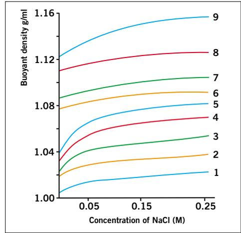
**Figure 13.** Effects of salt concentration on the recorded densities of Density Marker Beads in gradients of Percoll. Numbers refer to different bead types; the exact density of specific lots is printed on the box label. (Work from Amersham Biosciences, Uppsala, Sweden.)
