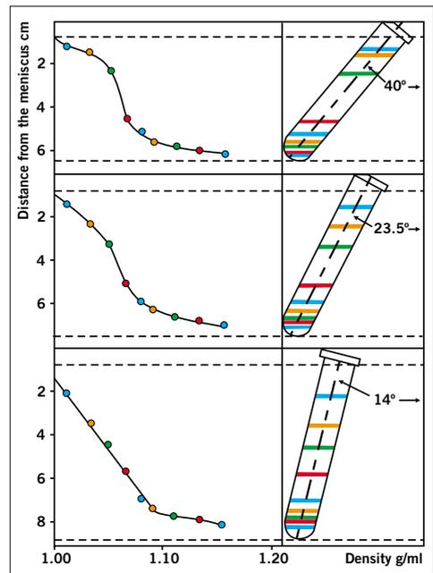
**Figure 8.** The effect of rotor angle on gradient development using Percoll. Starting density was 1.065 g/ml in 0.15 M NaCl. Running conditions: 30,000 x g for 14 minutes. Colored lines refer to the positions of the colored density marker beads. (45, reproduced by kind permission of the authors and publisher.)
