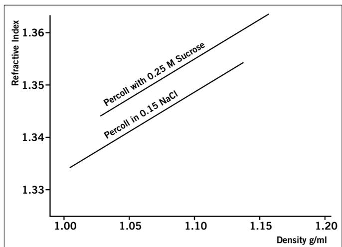
Figure 16. Refractive index as a function of density of a Percoll gradient. (Work from Amersham Biosciences, Uppsala, Sweden.)
