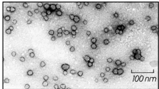
Figure 3. Electron microscopy of Percoll particles. Negative contrast with 1% uranyl acetate at pH 4.6 (21, reproduced by kind permission of the authors and publisher).
