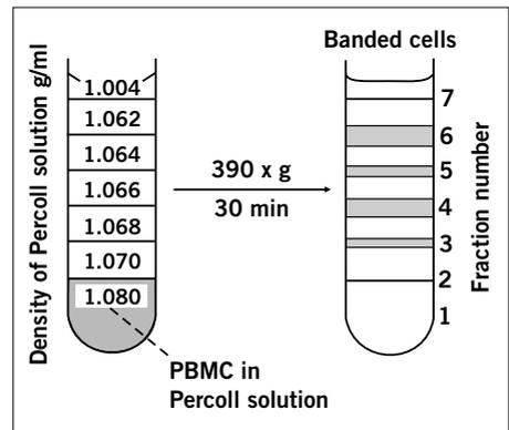
Figure 11. Separation of lymphocytes and monocytes by discontinuous density centrifugation in Percoll.  $1.5\text{-}2.0 \times 10^7$  PBMC (peripheral blood mononuclear cells) isolated on Ficoll Paque were mixed in 11.25 ml of Percoll in Hanks BSS containing 1% HEPES buffer (density = 1.080 g/ml) and underlayered below the steps shown in the figure (69, reproduced by kind permission of the authors and publisher).
