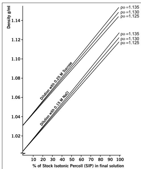
**Figure 5.** Dilution of Stock Isotonic Percoll (SIP) with iso-osmotic saline or sucrose solution.  $\rho_0$  is the density of the Percoll (undiluted). SIP is prepared as described on page 12. The calibration lines shown are for guidance only. For accurate density measurements, refer to the formula given in the text. (Work from Amersham Biosciences, Uppsala, Sweden.)
