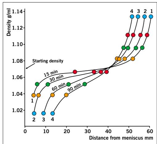
Figure 4. Isometric gradient formation by Percoll in an angle-head rotor, 8 x 14 ml (MSE Superspeed centrifuge) starting density 1.07 g/ml in 0.15 M NaCl. Running conditions: 20,000 x g for 15, 30, 60 and 90 minutes. Gradient density was monitored by means of colored Density Marker Beads. See Figure 12, page 23 (Work from Amersham Biosciences, Uppsala, Sweden).
