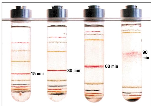
**Figure 12.** Banding of Density Marker Beads in gradients of Percoll as described in Figure 4. (Work from Amersham Biosciences, Uppsala, Sweden.)
